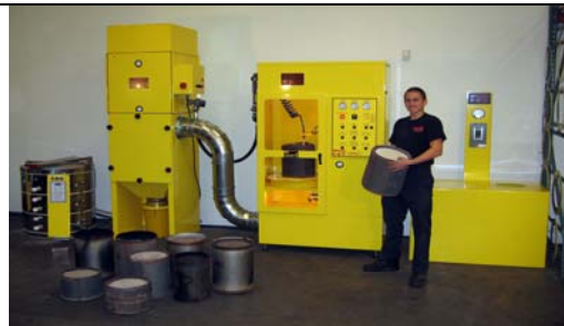
FSX Technology in Altoona Stage 1–Pneumatic using 'air knife' FSX technology Stage 2 – Optional thermal cleaning on-site
